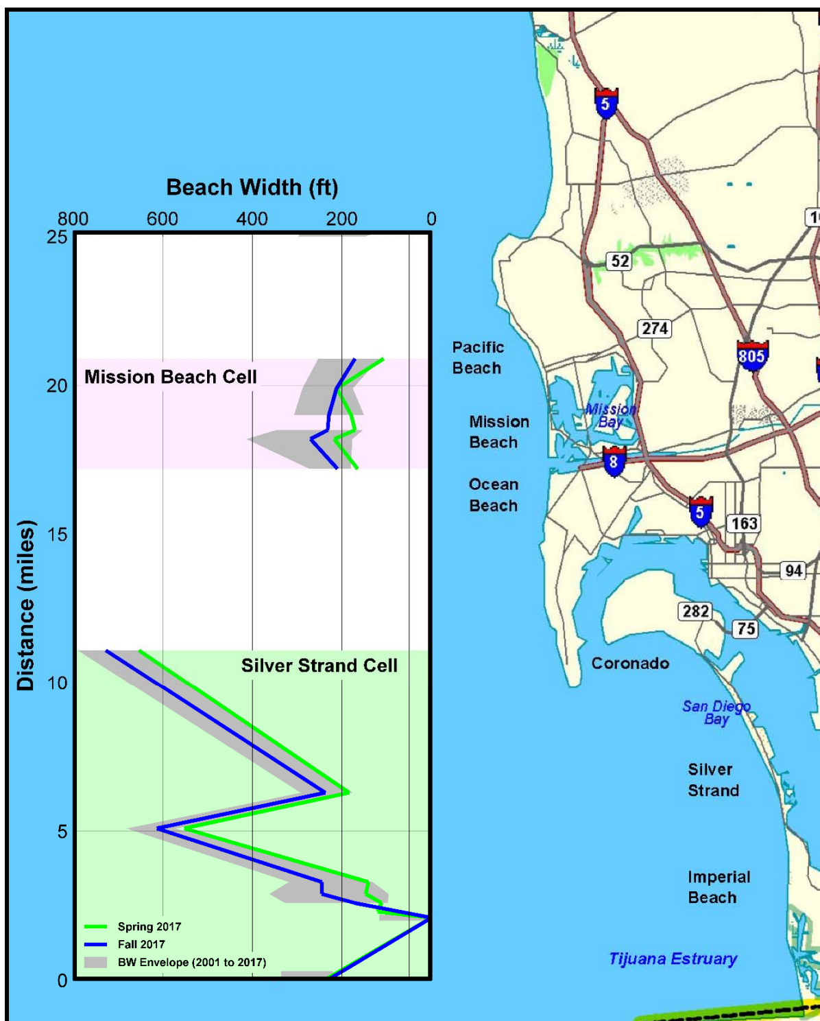
Figure 12a. Comparison of 2017 MSL Beach Widths with the Post-RBSP I Envelope in the Silver Strand and Mission Beach Littoral Cells
